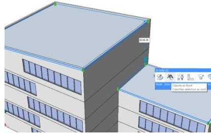
2. Classifying elements can be done manually, or automatically using **BIMIFY**
