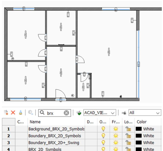
with the actual section, you need to use the **BRX\_2D+** layer. This is, for example, handy for doors, where you want to display a door swing together with the cut-through representation of the door.
