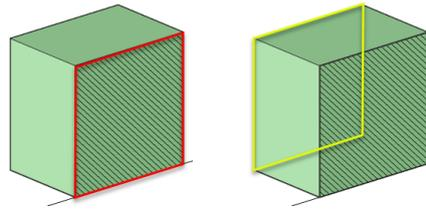
4. For the red object, only **one** layer will be created. Since the section plane does not cut through this object, only a **Background\_Layer2** layer will be created. Thus, the section result will look like the image shown here.
