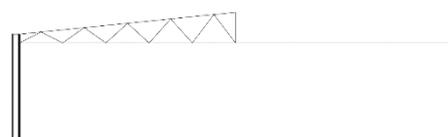
11. Select the truss pattern and upper line and bring up the **MANIPULATOR** (Quad: **Modify** tab). Drag the Manipulator to the right spot by using the little white grips. Stand on the little blue **Flip along X-axis** icon and flip the truss.
